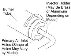
Figure 26 - Injector Holder On Outlet Burner Tube
